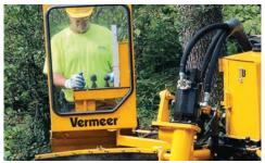
**OPERATOR PRESENCE SYSTEM.** This user-friendly operator system is intended to help protect the operator and enhance operator safety. If the operator's hand(s) leave the controls for more than one second, the cutter wheel will disengage, come to a stop and the cutter wheel indicator light will go out.
