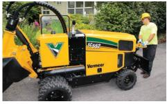
**AUXILIARY CONTROL STATION.** In narrow jobsite conditions that restrict use of the main control station, the operator can control ground drive and steering functions from this folding station mounted at the front end of the machine.
