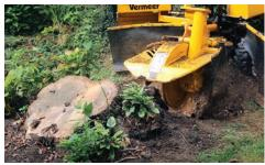
MAXIMUM CUTTING WIDTH. The SC552 reduce the operator's time repositioning the machine with a cutting height of 31" (78.7 cm) above ground and 25" (63.5 cm) below grade. the straight-line cutting dimension allows the operator to cut a 6' (1.8 m) stump without repositioning the machine.
