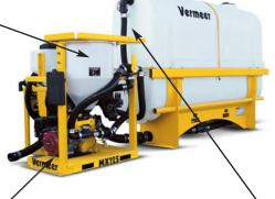
**Choice of engine.** The MX125 is available with either a 5.5-hp (4.1-kW) Honda gas engine or 6.7-hp (5-kW) Hatz diesel engine. **Modular design.** Flexible setup allows the power pack to be mounted on either end of the tank or trailer for accessibility and customer preference.
