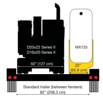
**Narrow profile.** The MX125 [500-gal (1892.7-L) option only] features a narrow profile for ease of side-by-side trailer transport with a horizontal directional drill.
